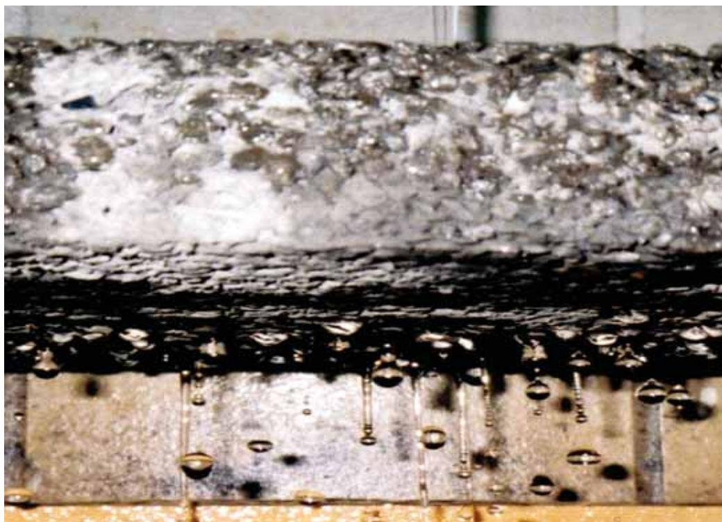
Picture taken in laboratory: draining effect of a Mapedrain Mortar 's sample
