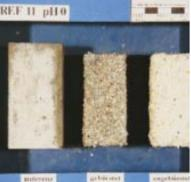
Reference mortar according to the "Directives for controlling mortars used in sewage pipes"
