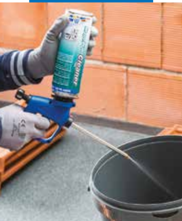
Cleaning a foam filler extrusion gun
