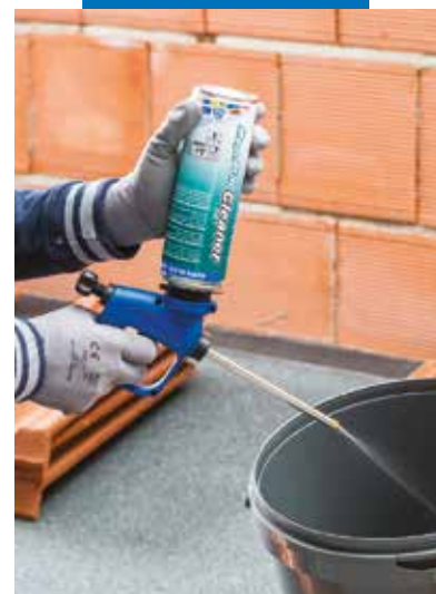
Cleaning a foam filler extrusion gun
