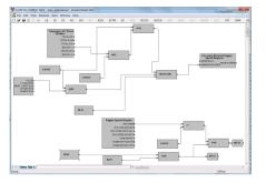
The EMCP programmable logic software package is a PC based program configuration which allows the of the programmable logic blocks, and is capable of running on a Windows based operating system. The programmable logic software allows the user to configure logic to change the operation of the EMCP control and interfaces within a limited scope.
