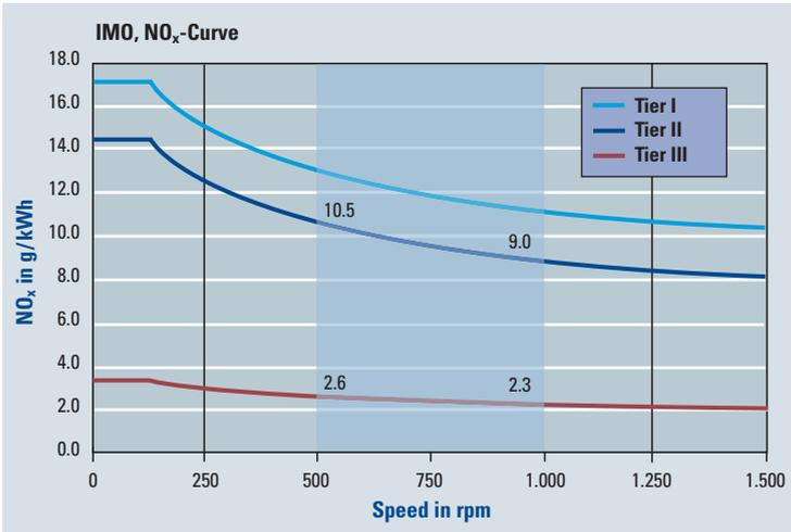
IMO Tier III regulations went into effect in 2016 and is valid for newly built vessels. The IMO Tier III regulations lower the permissible NO<sub>x</sub> emissions in NO<sub>x</sub> Emissions Control Areas (NECA) by about 75% in comparison to IMO Tier II. Outside of the NECA IMO Tier II remains valid.
