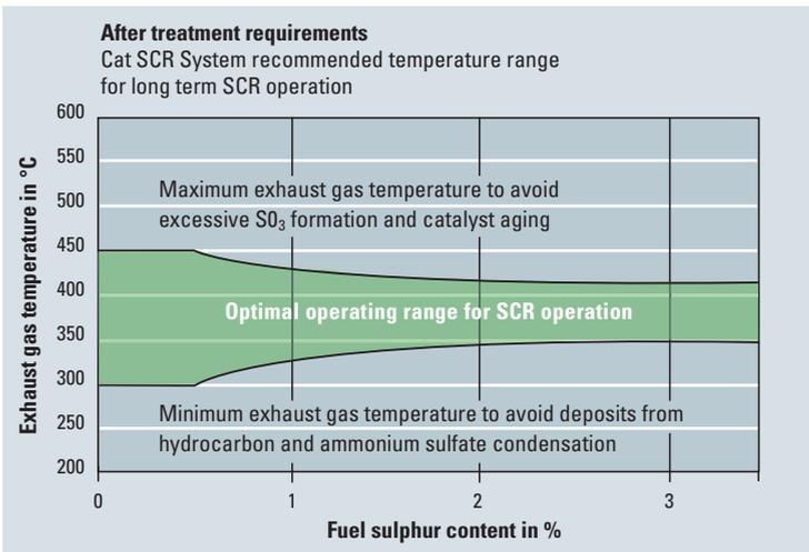
To avoid deposit buildup and ensure optimal operation of the SCR module, the exhaust gas temperature has to be adjusted to the operating conditions for each application.
