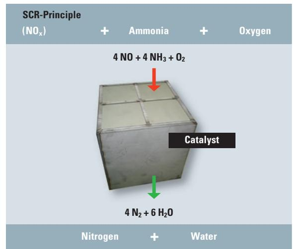
The Cat SCR System is based on selective catalytic reduction technology. A urea solution is injected into the hot exhaust gas and transformed to NH<sub>3</sub> and CO<sub>2</sub>. Inside the SCR module the NH<sub>3</sub> reacts with the NO<sub>x</sub> to form harmless nitrogen and water vapor, which are major components of ambient air.
