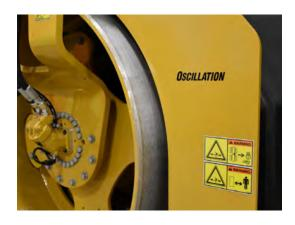
The design combines high-performance vertical vibration on the front drum with oscillation technology on the rear drum. The front drum with vertical vibration is available in two amplitude, five amplitude, or Versa-Vibe systems that provide initial compaction, while the rear drum with oscillation continues the excellent performance for optimal smoothness and density.
