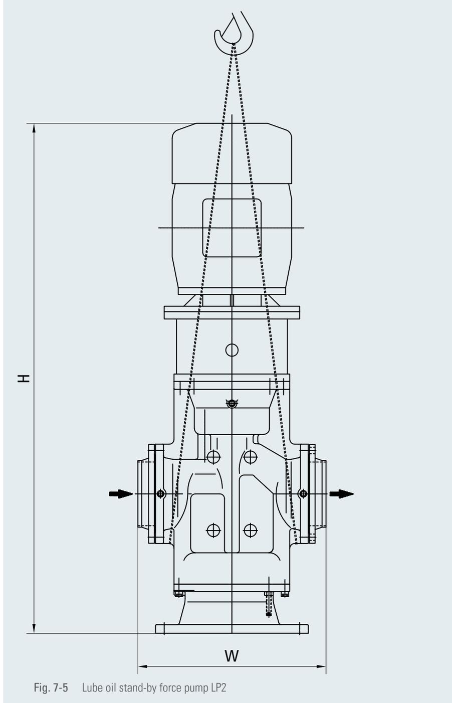
Fig. 7-5 Lube oil stand-by force pump LP2
