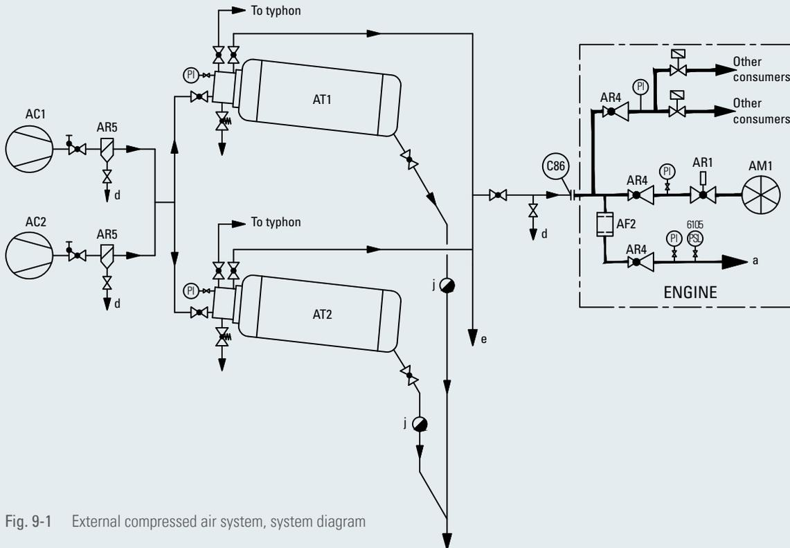
Fig. 9-1 External compressed air system, system diagram
