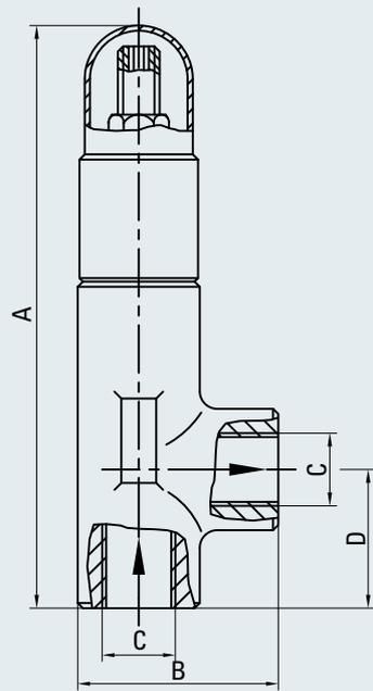
Fig 5-16 Fuel pressure regulating valve
