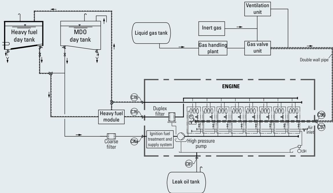
Fig. 6-1 Gas system diagram
