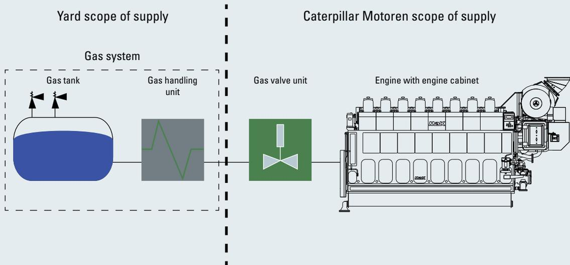
Fig. 13-6 Basic overview: dual fuel engine gas system
