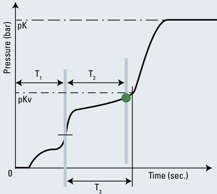
Fig. 13-7 Clutch in procedure for propulsion systems
