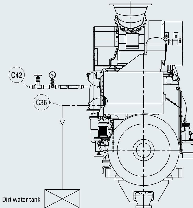
Fig. 11-8 Connection points fresh water and drain
