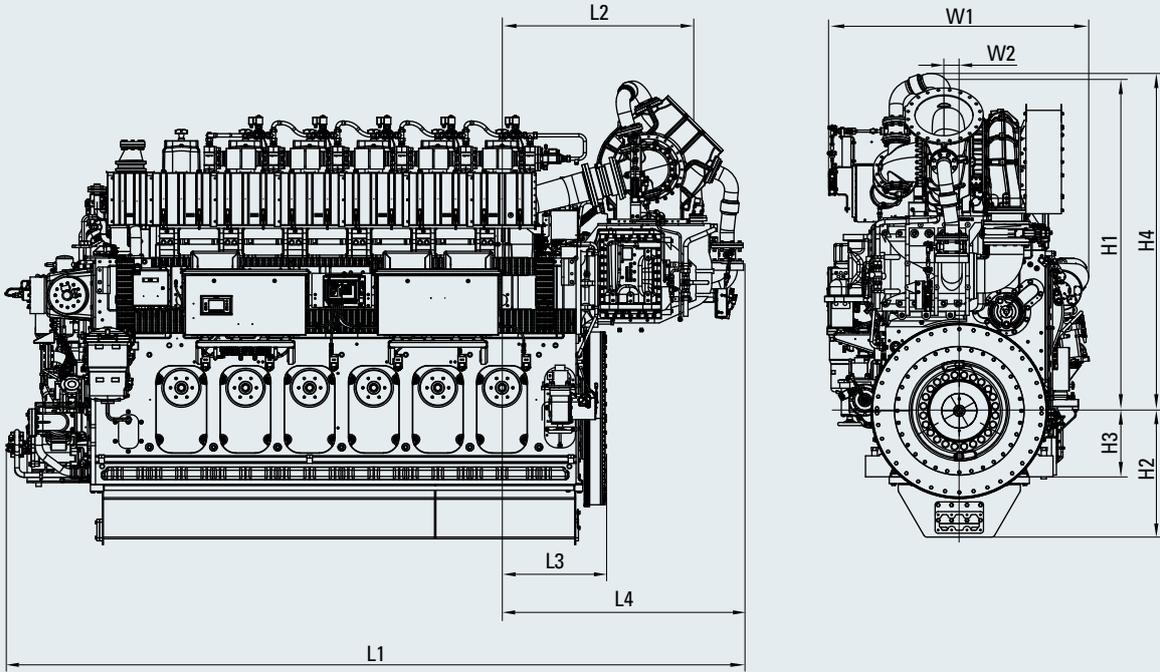
Fig. 2-2 Turbocharger at driving end – exhaust side
