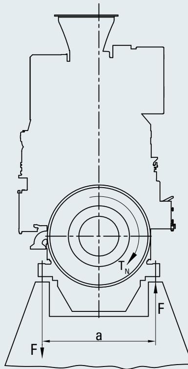
Fig. 15-1 Static load
