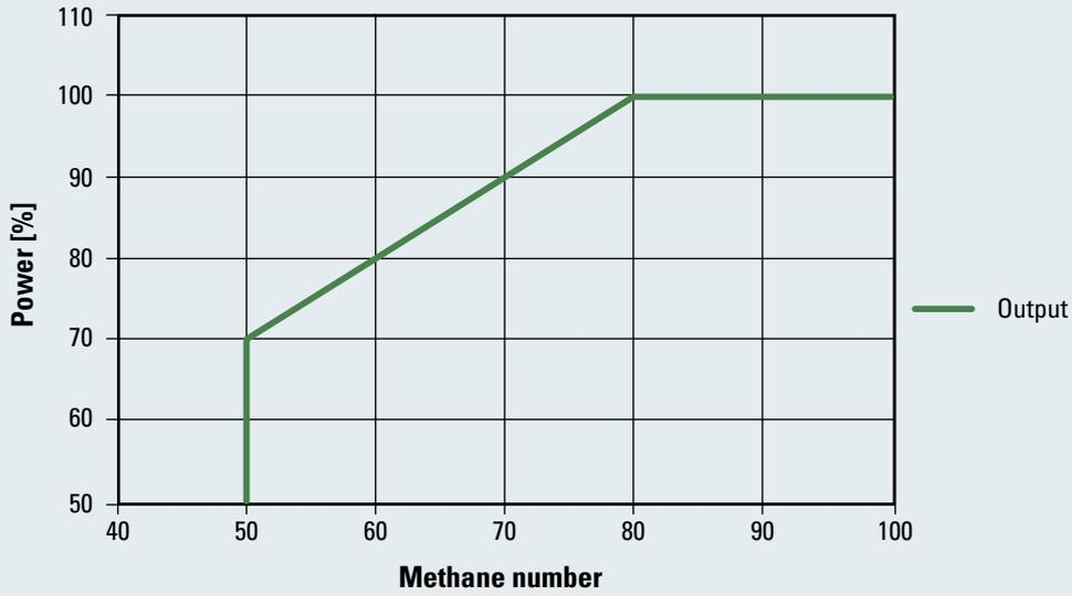
Fig. 3-7 Power as function of methane number
