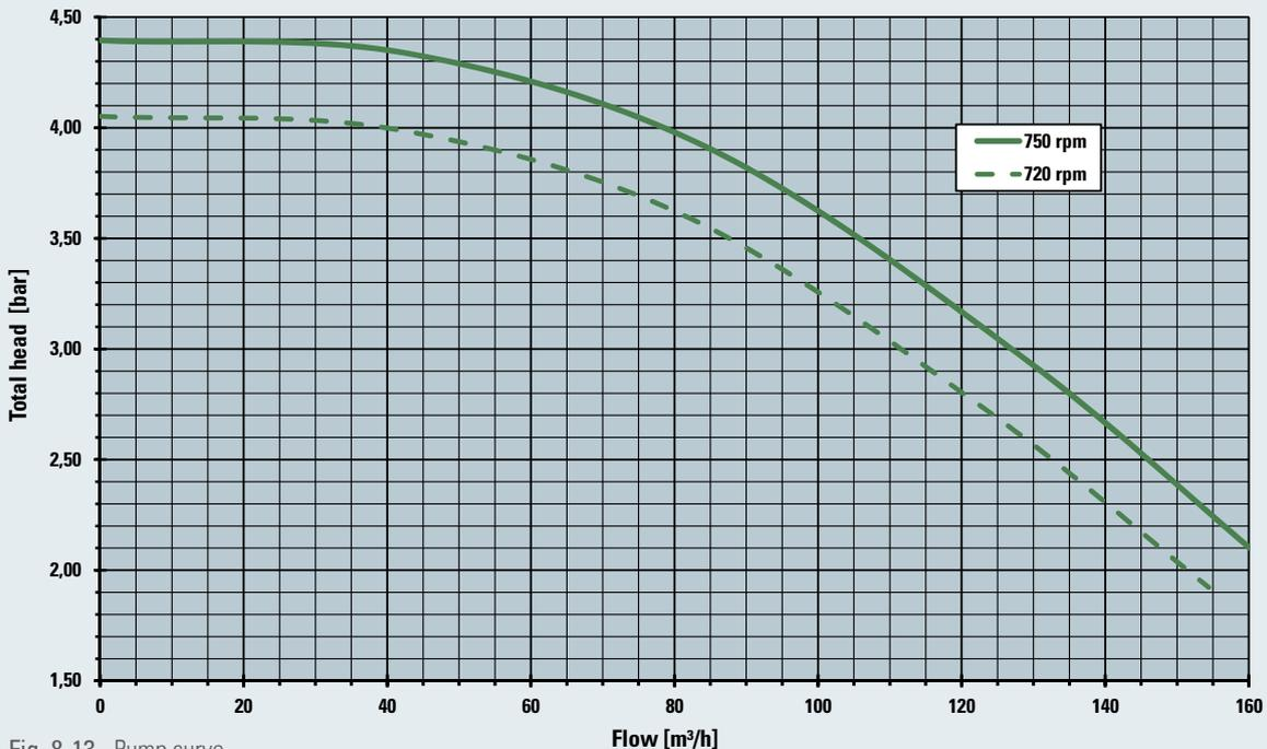
Fig. 8-13 Pump curve
