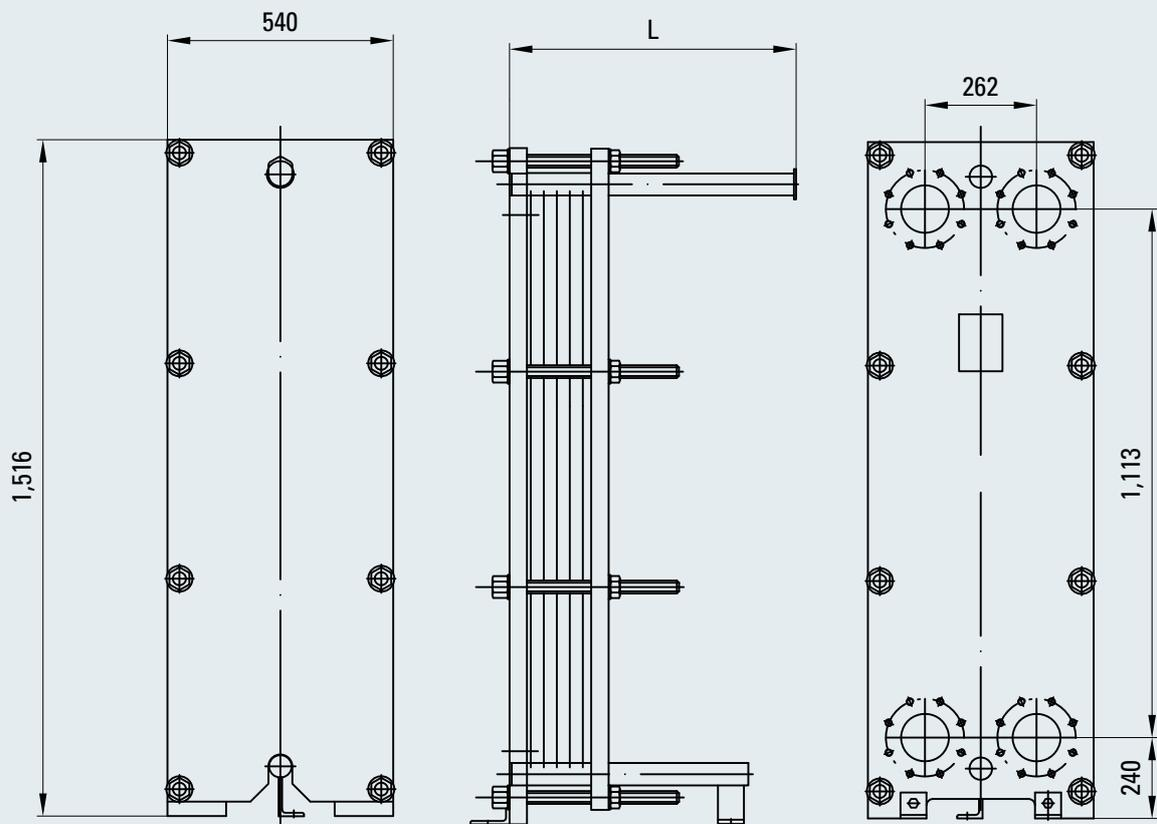
Fig. 7-8 Lube oil cooler LH1
