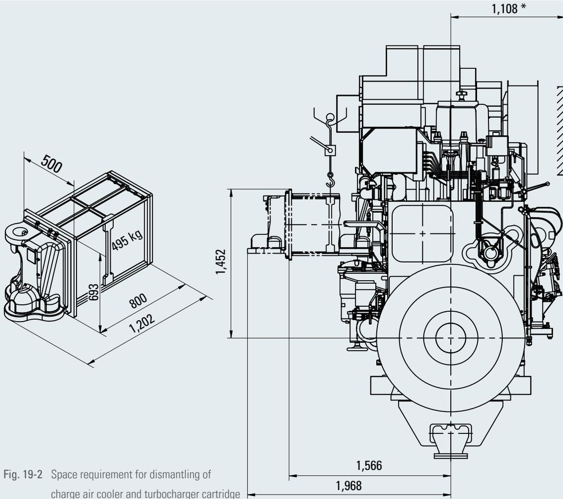
Fig. 19-2 Space requirement for dismantling of charge air cooler and turbocharger cartridge
