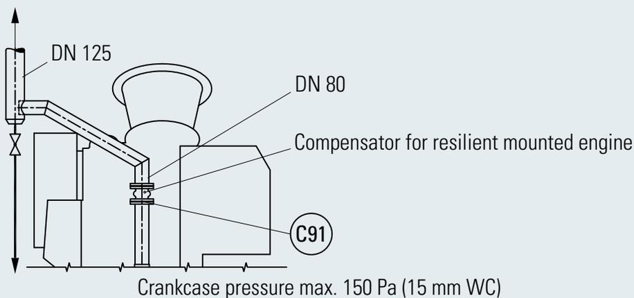
Fig. 7-14 Crankcase ventilation
