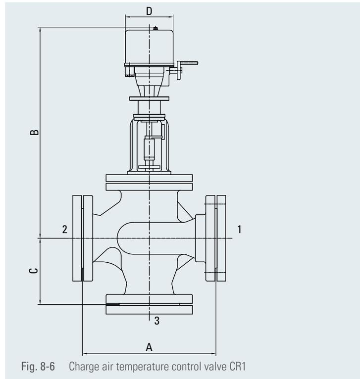
Fig. 8-6 Charge air temperature control valve CR1
