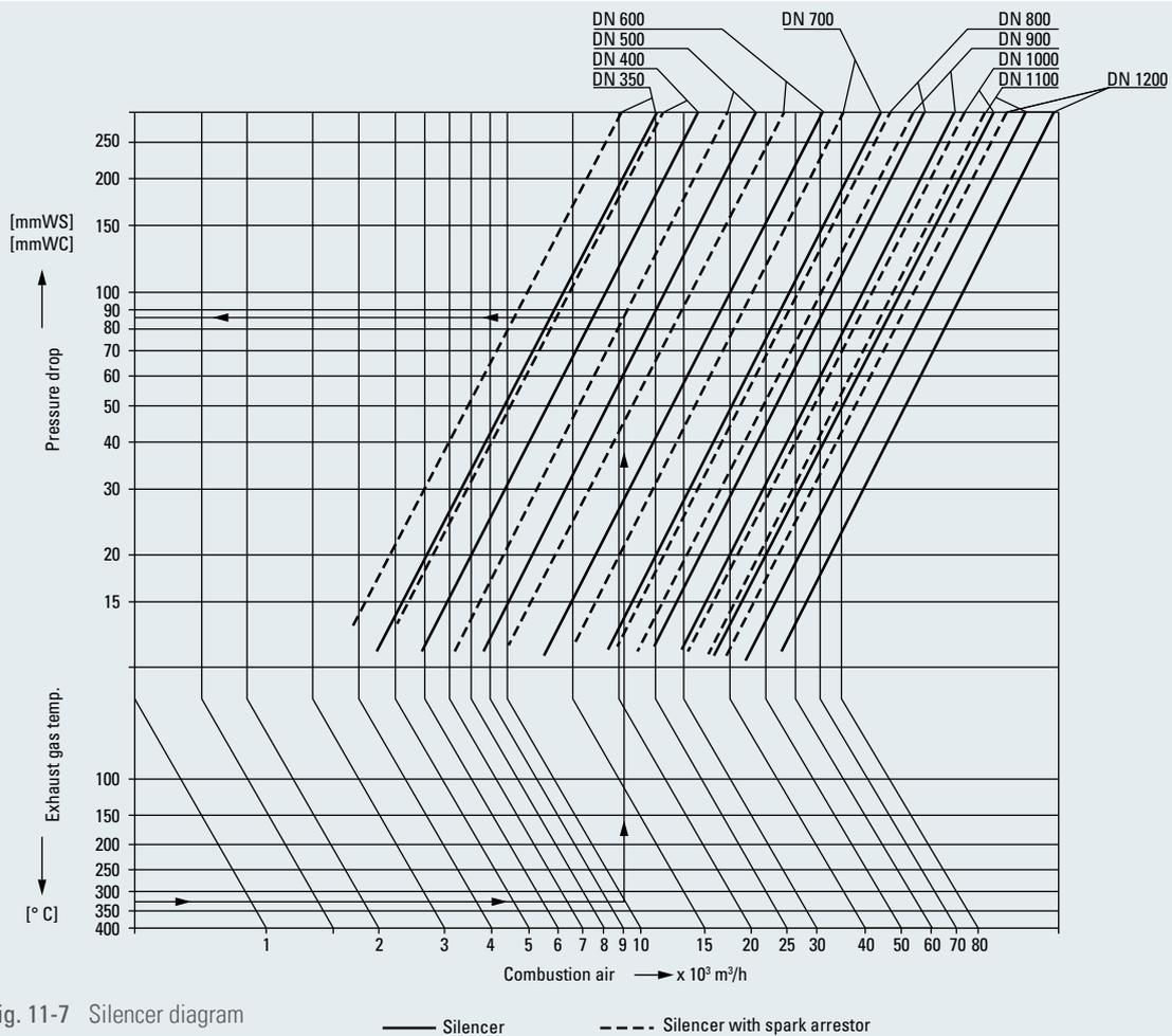
Fig. 11-7 Silencer diagram
