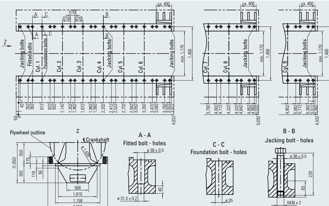
Fig. 14-1 Dimension of foundation dry sump pan
