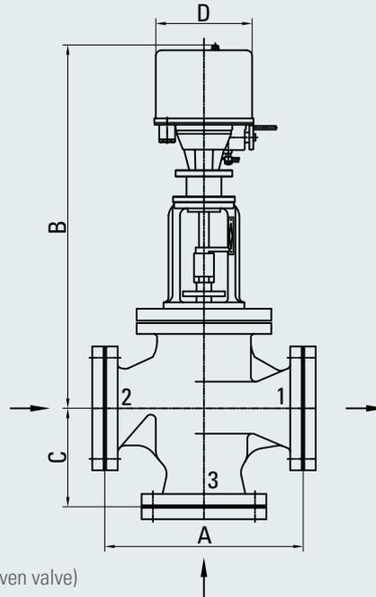
Fig. 7-10 Lube oil temperature control valve LR1 (electric driven valve)
