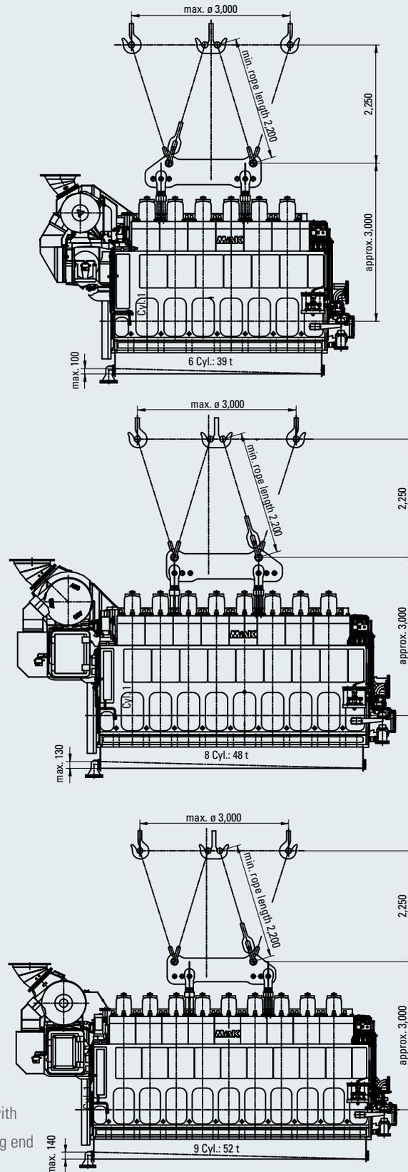
Fig. 21-2 Transport of engine with turbocharger at driving end
