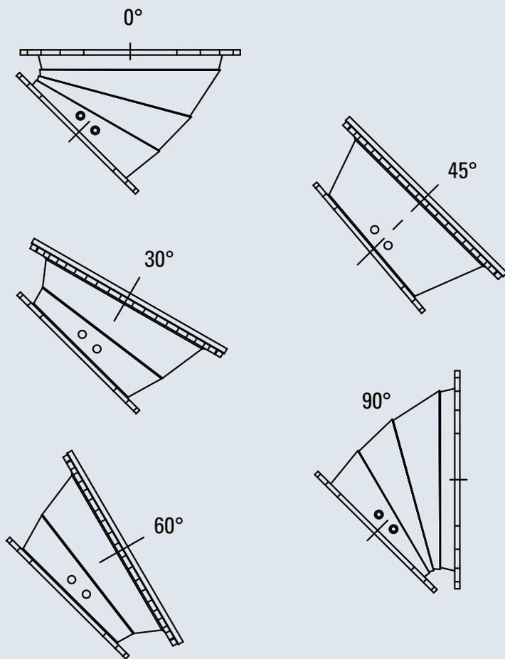
Fig. 11-2 8/9 M 34 DF nozzle orientation
