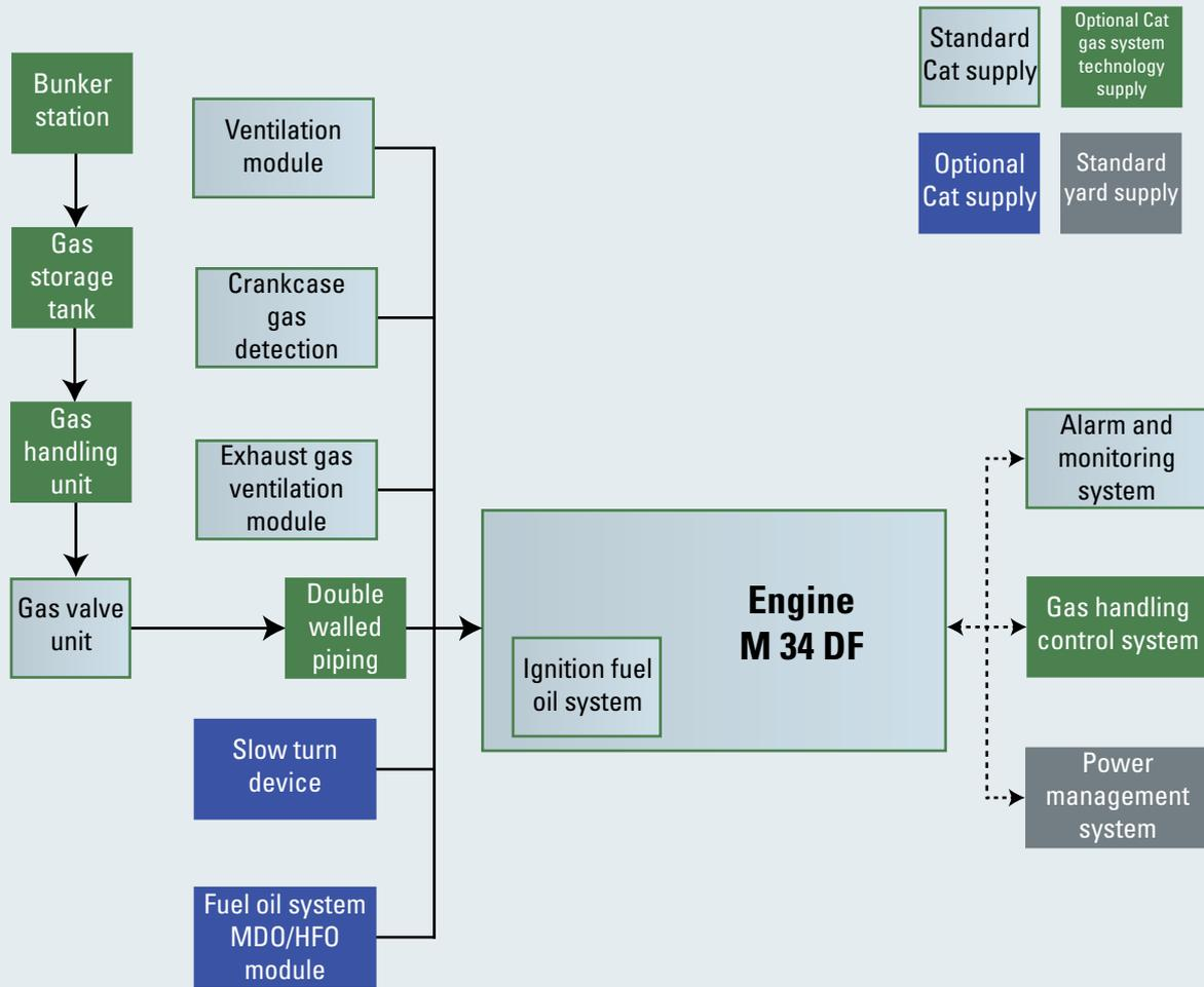
Fig. 24-1 Scope of supply M 34 DF Gas systems technology – block diagram
