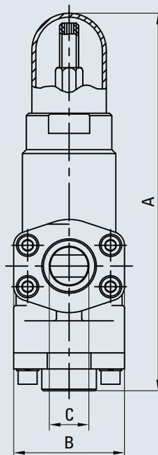
Fig 5-17 Fuel pressure regulating valve
