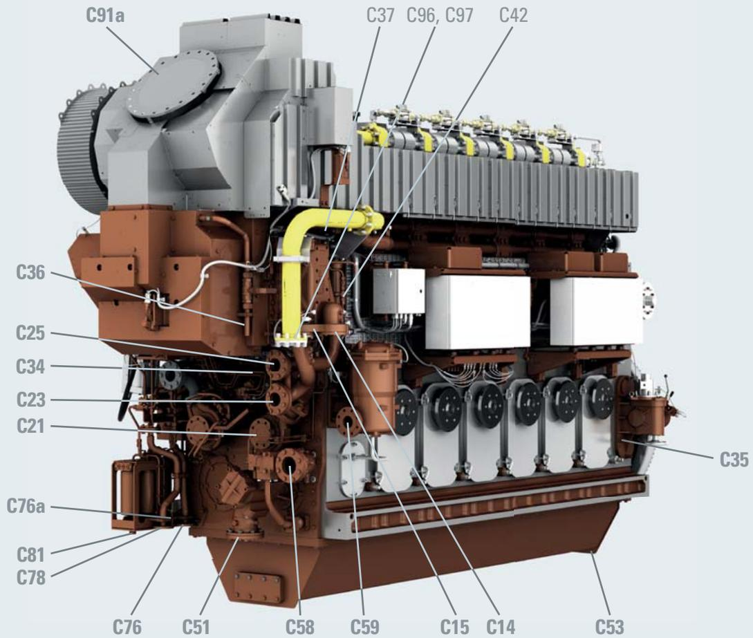
Fig. 2-3 Connecting points at the engine
