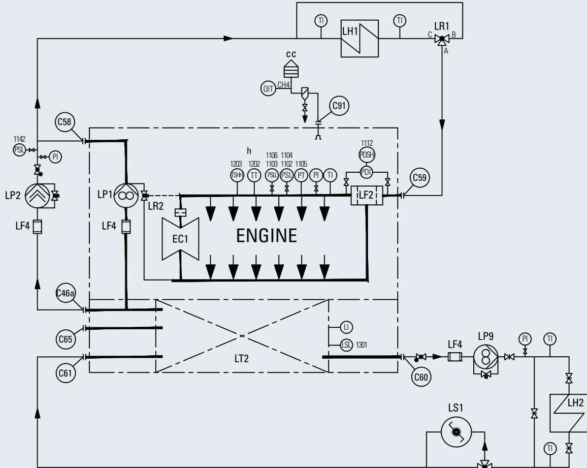
Fig. 7-11 System diagram, wet sump tank
