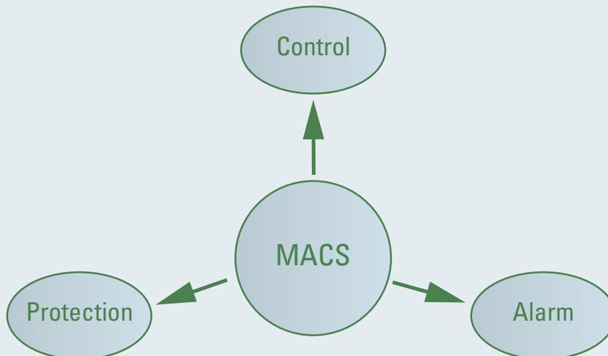
The M 34 DF engines will be provided with a new Modular Alarm and Control System, called MACS. The basic engine control and monitoring system will be installed in the local control panel. Where extension modules are necessary external plc based I/O extension modules will be installed.
