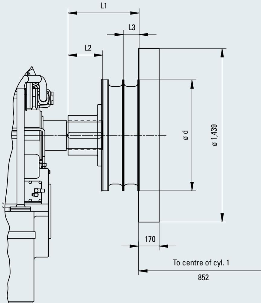
Fig. 17-1 Flywheel and flexible coupling
