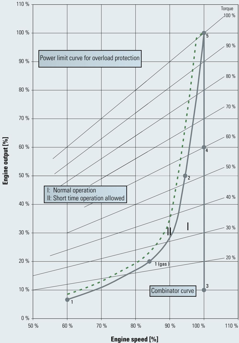
Fig. 3-1 CPP operation - diesel and gas mode
