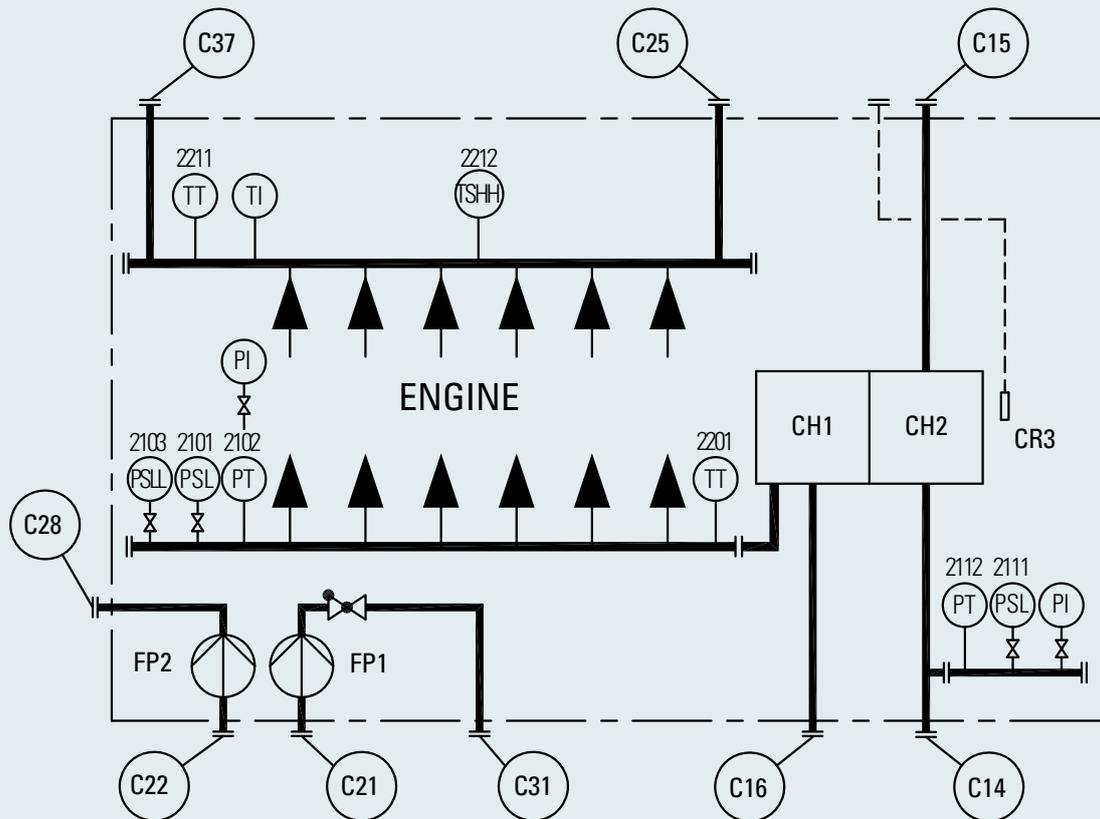
Fig. 8-1 Internal cooling water system, system diagram, turbocharger at driving end
