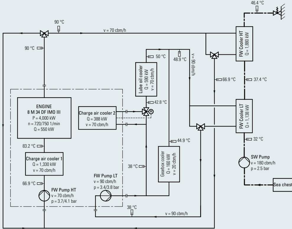
Fig. 8-10 Heat balance, system diagram 8 M 34 DF
