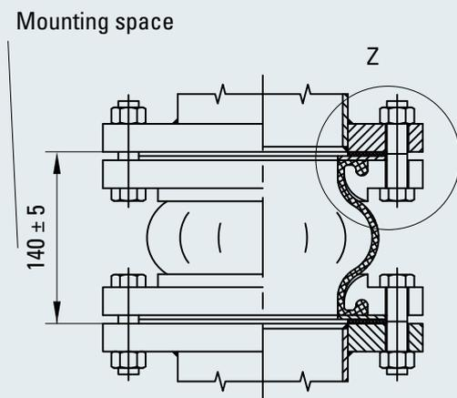
Fig. 18-1 Rubber expansion joint
