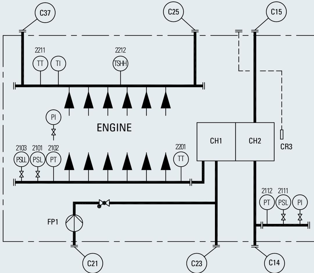
Fig. 8-2 Internal cooling water system, system diagram, turbocharger at free end
