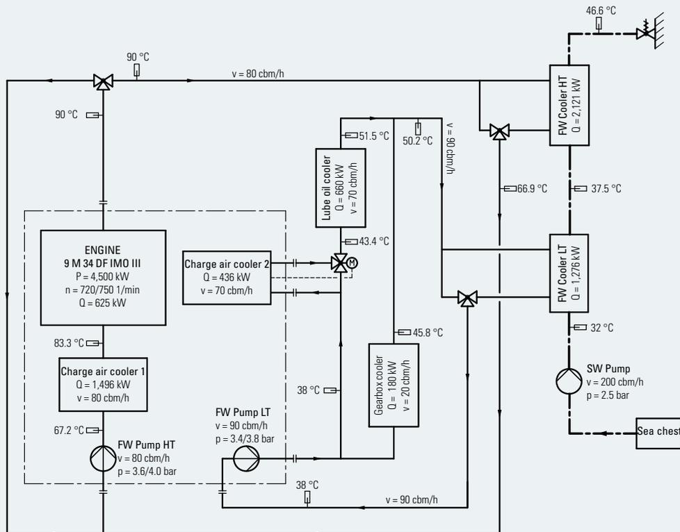
Fig. 8-11 Heat balance, system diagram 9 M 34 DF
