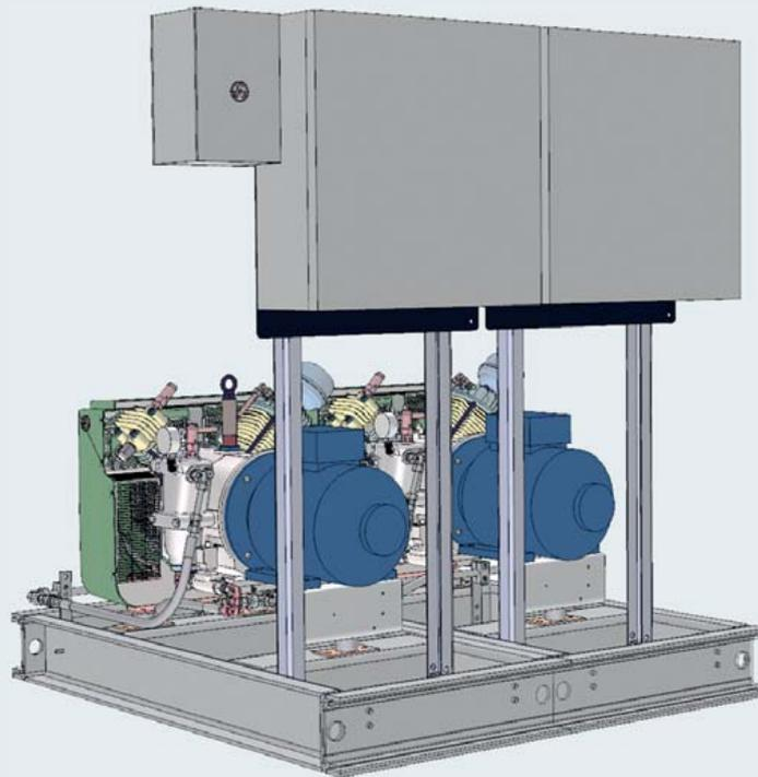
Fig. 9-2 Compressor AC1, AC2
