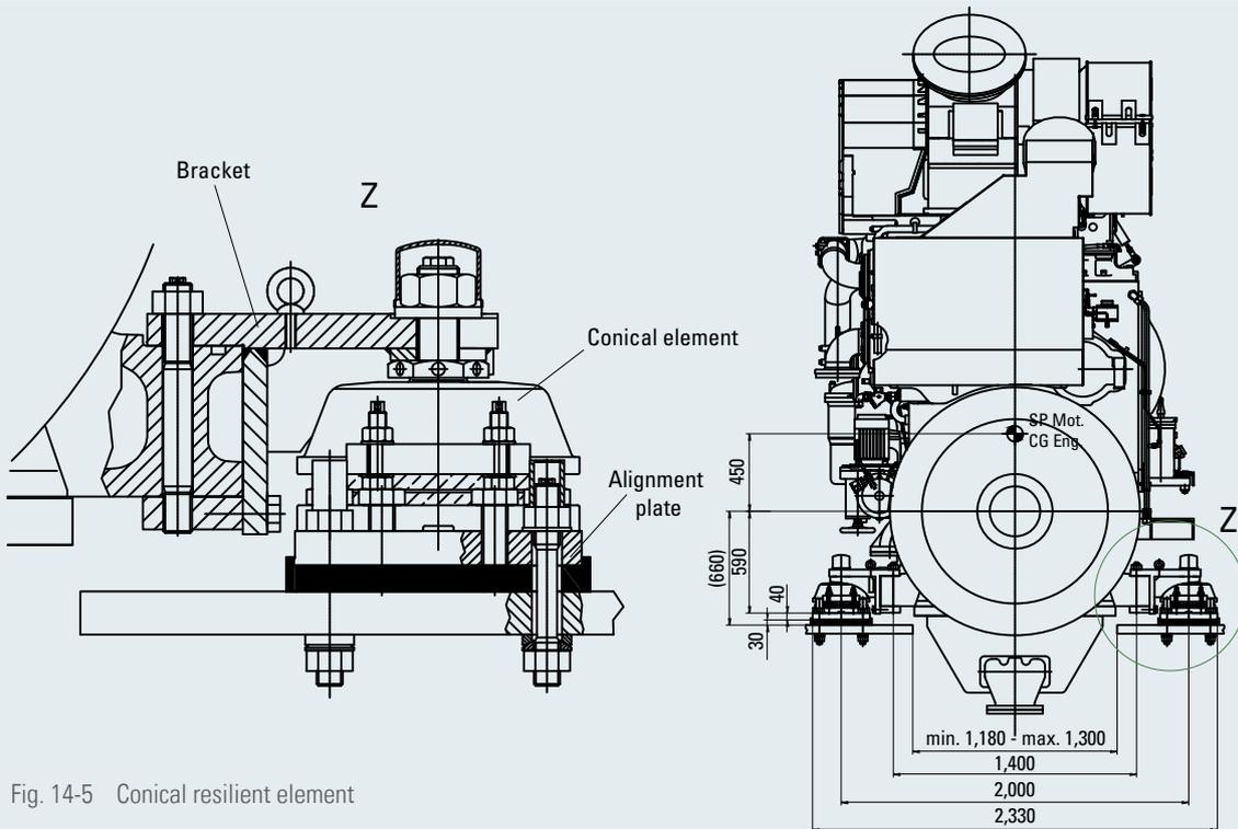
Fig. 14-5 Conical resilient element
