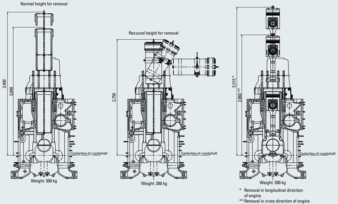
Fig. 19-3 Removal of piston and cylinder liner
