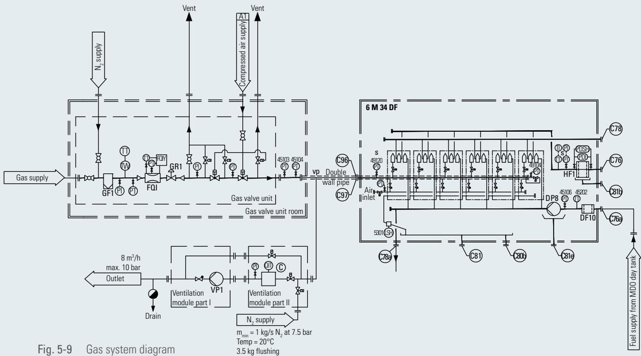
Fig. 5-9 Gas system diagram
