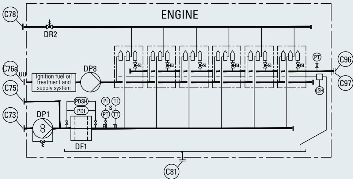
Fig. 5-1 Internal fuel oil system, system diagram
