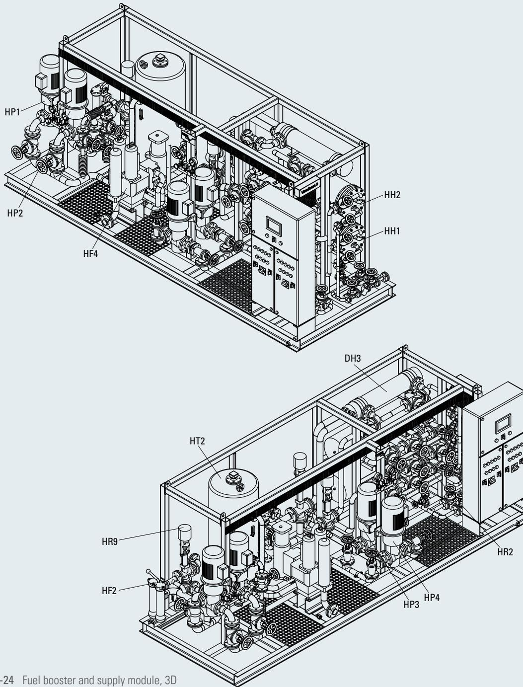
Fig. 5-24 Fuel booster and supply module, 3D
