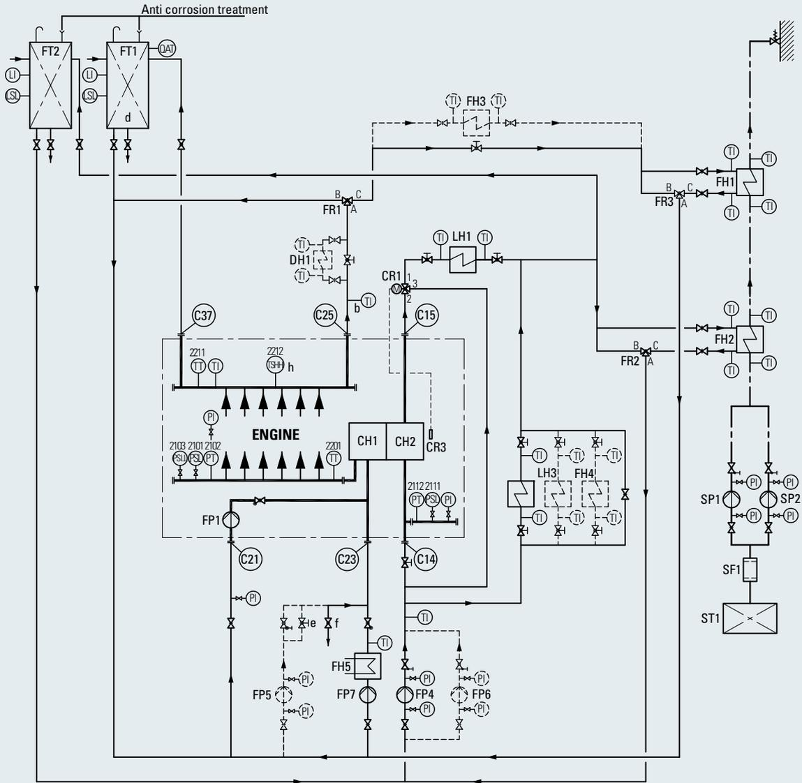
Fig. 8-4 External cooling water system, system diagram, turbocharger at free end
