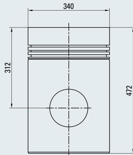
Fig. 21-7 Piston, weight 97.6 kg
