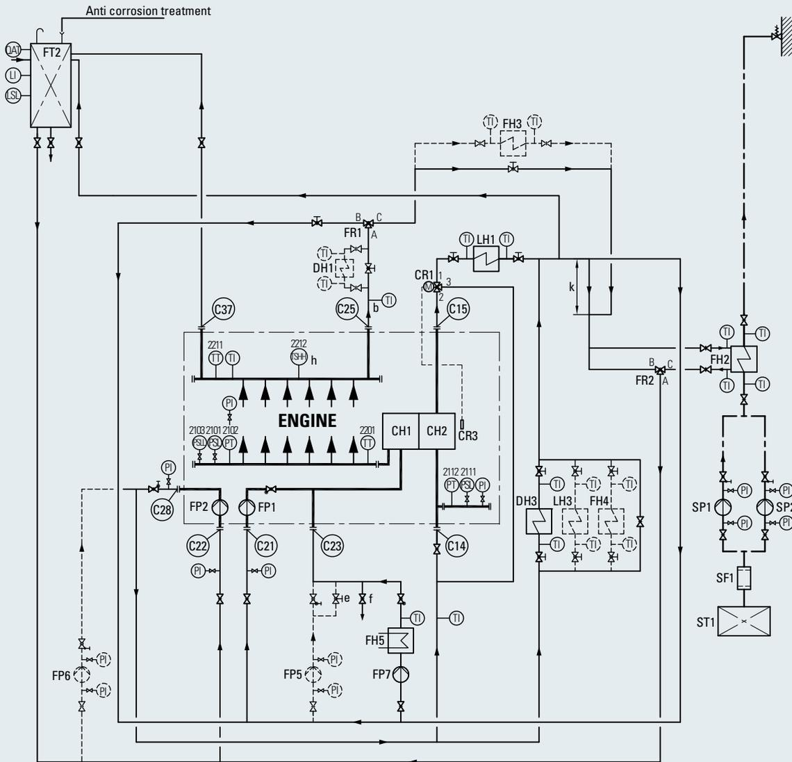
Fig. 8-5 Secondary circuit cooling system, system diagram, turbocharger at free end
