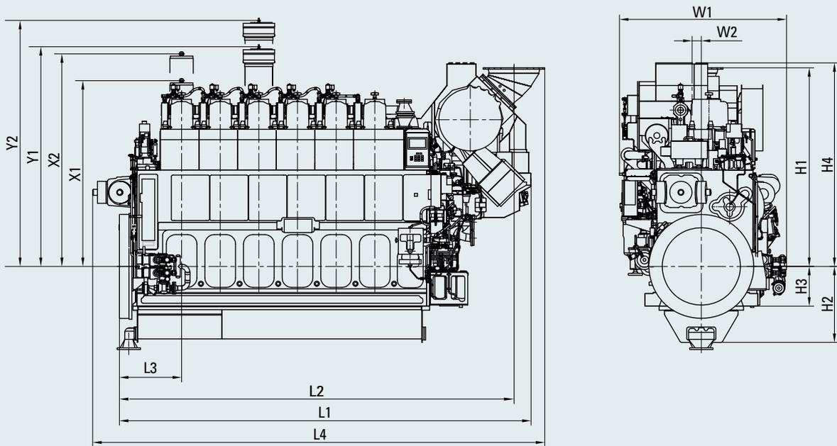
Fig. 2-1 Turbocharger at free end – control side
