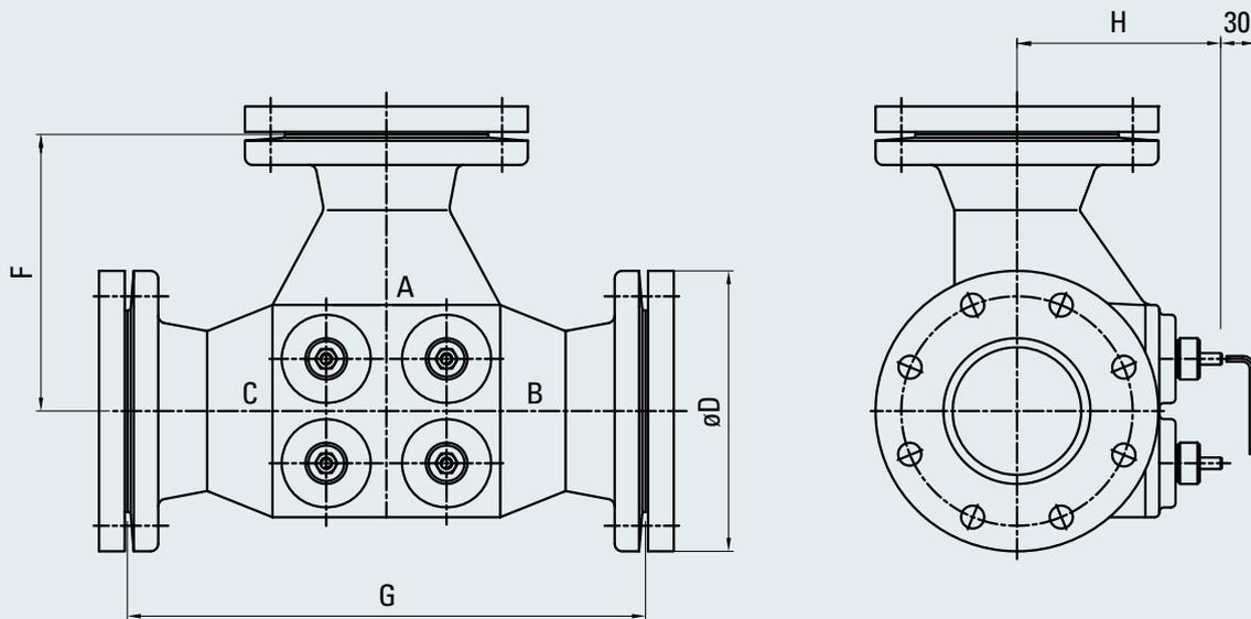
Fig. 7-9 Lube oil temperature control valve LR1
