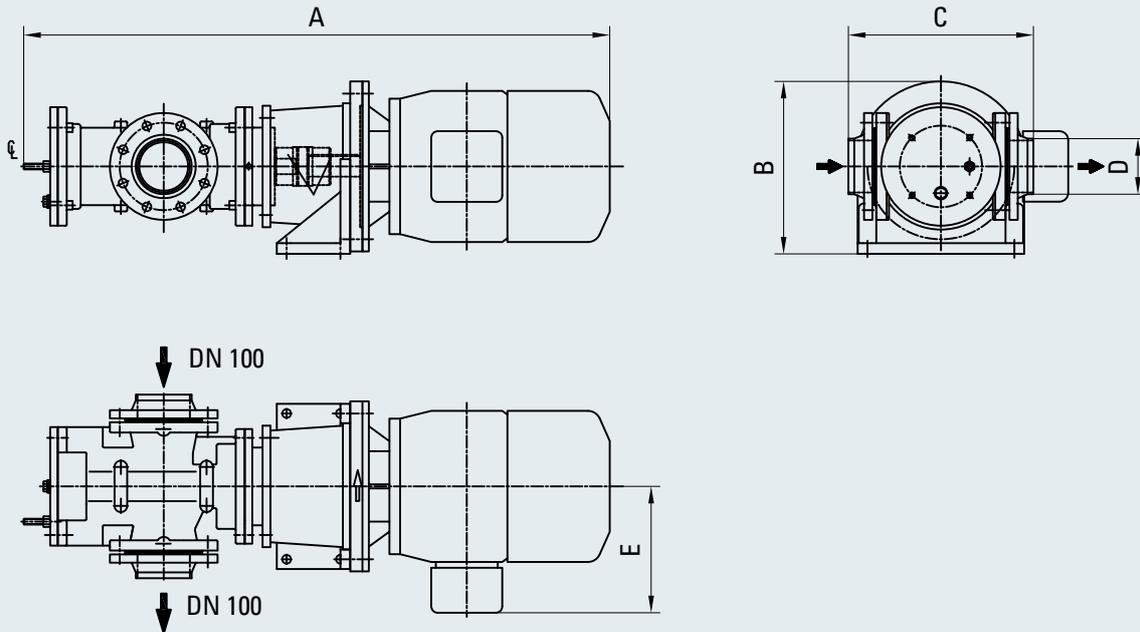
Fig. 7-6 Prelubricating pump LP5
