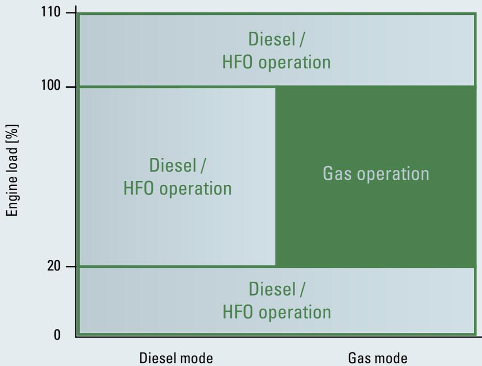
Fig. 3-5 Load restrictions in gas mode
