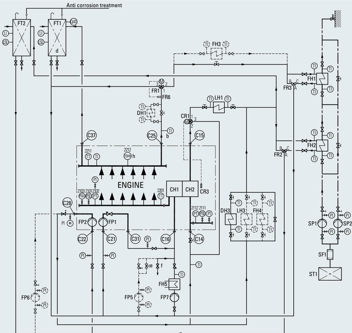
Fig. 8-3 External cooling water system, system diagram, turbocharger at driving end
