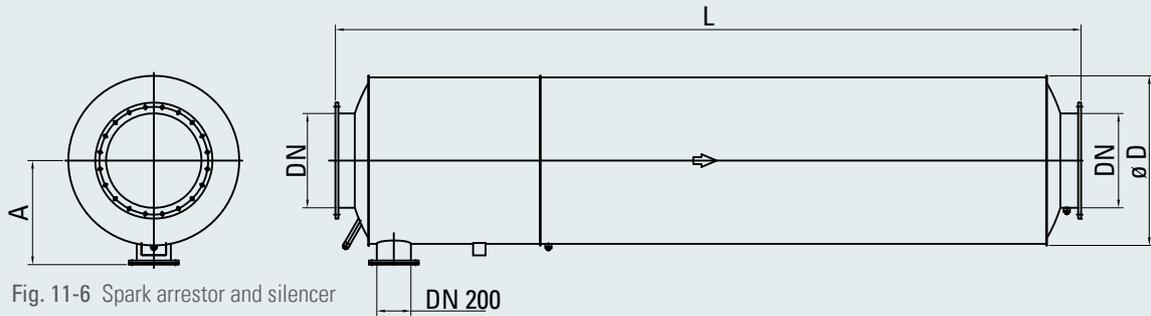
Fig. 11-6 Spark arrestor and silencer
