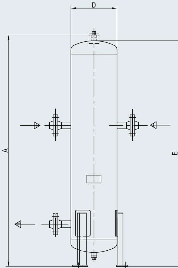
Fig. 5-19 Mixing tank HT2
