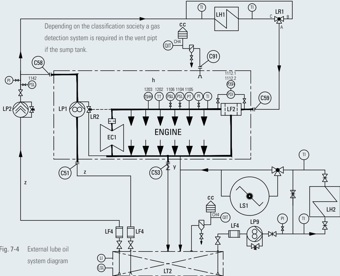
Fig. 7-4 External lube oil system diagram
