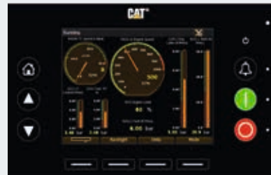
Fig. 11-10 DCU (display and alarm system)
