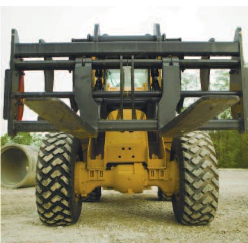
A new, open coupler frame design opens sight lines from the operator's seat, making it easier than ever before to engage and disengage work tool with certainty.
