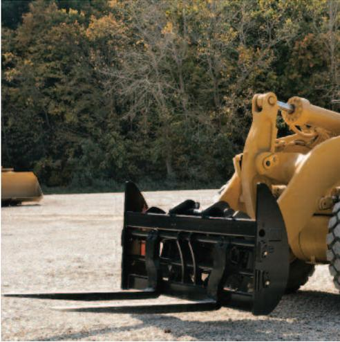
Forks are essential tools on any job site. Unload trucks, place material and load up again.
