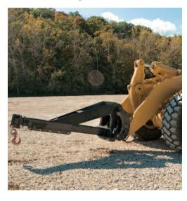
Material Handling Arms precisely place pipe, concrete blocks, highway dividers and other construction materials quickly — with maximum visibility and control. They provide superior performance when compared to chains-on-buckets or other improvised means. With a Material Handling Arm, the operator has full view of the load, job site and other workers. Work is faster, more efficient and more safe.
