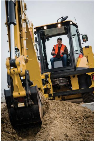
The 428F2 is fitted with mechanical controls providing low effort operation, with the ability to choose between ISO (Excavator) or SAE (Backhoe) control patterns. Providing easy and safe operation for operators of any experience or ability.
