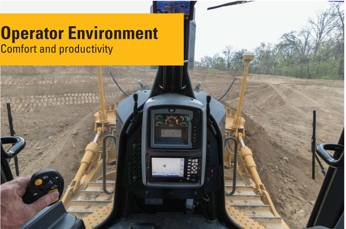
The D7E features a quiet, spacious cab. The center-post design gives you outstanding visibility all around the machine to help operators work more confidently and safely. Operators can also enjoy added comforts like manually adjustable armrests and a heated/ventilated seat option.
