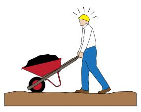
The wheelbarrow tire sinks into loose soil, requiring greater effort to push it through.
