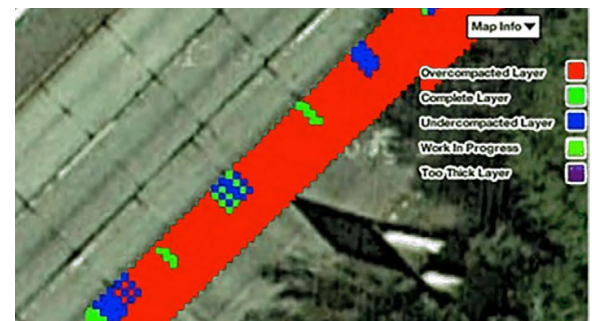
Compaction Meter Value (CMV) can help indicate road structure health on "Mill and Fill" applications
