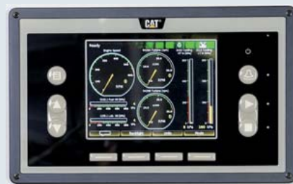
Fig. 11-7 DCU (display and alarm system)
