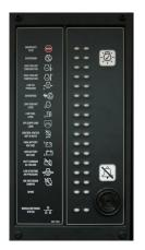
The EMCP 4 CAN Annunciator serves to display generator set system alarm conditions and status indications. The annunciator has been designed for use on the accessory communication network and may be used in either local (package mounted) or remote (up to 800 feet) application. A maximum of four annunciators may be used with a single EMCP 4.3
