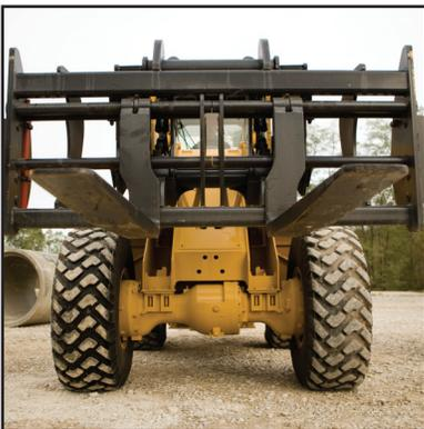
A new, open coupler frame design opens sight lines from the operator's seat, making it easier than ever before to engage and disengage attachments with certainty.
