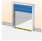
A set of a photocell transmitter with reflector or receiver is installed in the door opening. If the photocell beam is interrupted during closing, the door will stop in less than 30mm and reverse to the fully open position. Installed in the door opening.
