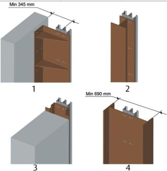
1. Fitting against wall. 2-4. Fitting in opening.
