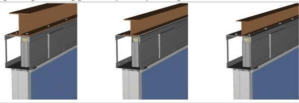
Fitting in door opening (header box screwed, welded or fixed beam clamps).
