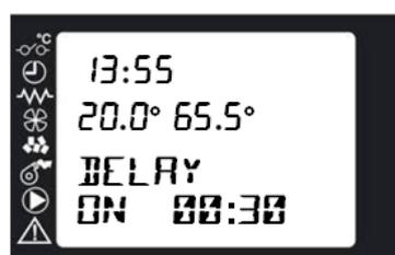
With DELAY ON (or OFF) set, the main screen displays the time countdown until the set switch-on (or shutdown). The appliance can be switched on (or shutdown) at any time even in this situation by using the normal procedure.
