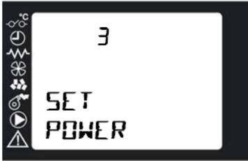
To change the operating output, press Key **5** on the main page to immediately open the screen where you can use the Keys 5 or 6 to select from the five settable output settings. After selecting the required output level, press Key **3** to return to the main page.
