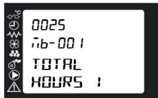
will indicate that the device has operated for a total of 10025 hours.
