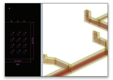
Duct bank spacers configuration is used to define spacing between conduits. Concrete envelope is wrapping selected conduits into duct bank. Cables are auto routed through duct banks and manholes.
