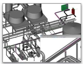
The 3D modeling software allows manual and automatic cable routing based on user-definable constraints.
