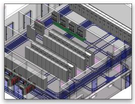
With Bentley Raceway and Cable Management, users can place raceways and electrical equipment to create a comprehensive design.
