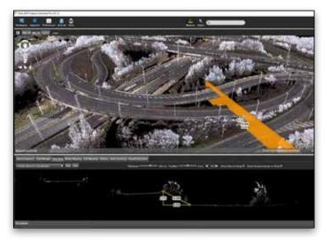
Orbit 3DM Feature Extraction allows you to efficiently measure, extract, and detect assets. You can process cross-sectionsalong the trajectory, create a profile along a 3D path, calculate mapping data and analyze volumes over time, export views and features, and create accurate reports.
