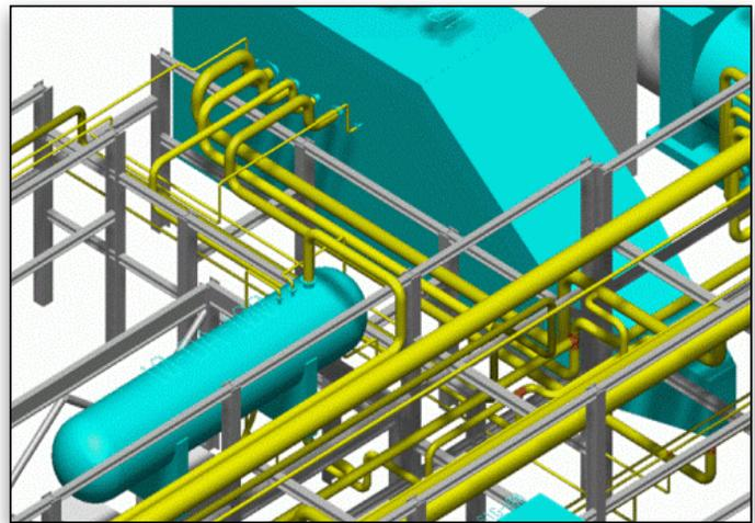
*Rule-based AutoRouter lays out pipe using pipe designer’s preferences while avoiding obstacles on the pipeway.*
