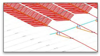
Automatic rule-based design of draped stope panels and ledges on reef enables substantial time savings during layout.
