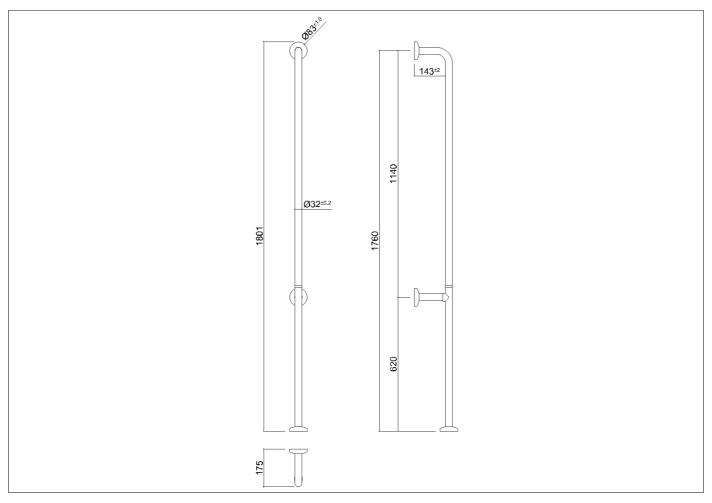
Wall-to-floor grab bar made of steel pipe, painted with synthetic thermoplastic powder of plant origin, Rilsan®
