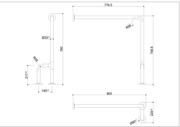
90° wall-to-floor grab bar made of zinc-plated steel pipe, coated with biocompatible and warm-to-the-touch vinyl
