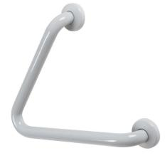
Safety corner grab rail 45° Ø 33 mm with antislip, vinyl coating and zincplated steel internal pipe without junctions. Active and long lasting antimicrobial
