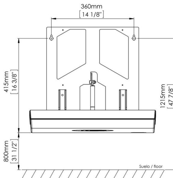
Following the above scheme, using the pencil, mark on the wall the top two holes of the changing station's holding structure. It is very important to make sure that the locations marked with the pencil for the mounting holes are at the same level before drilling the holes.
