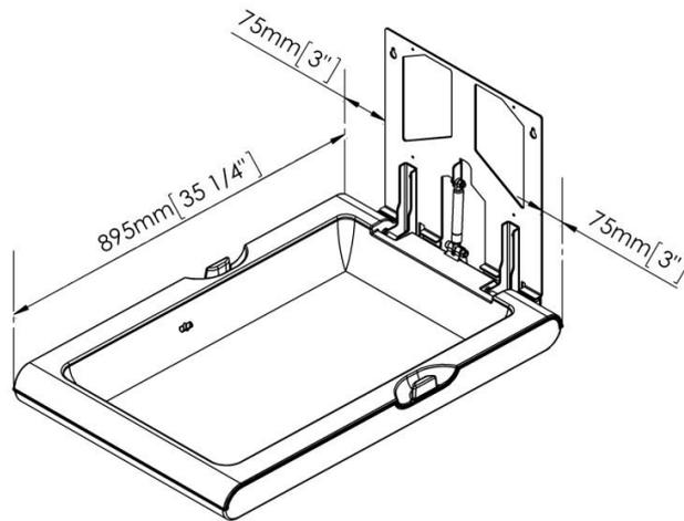
The recommended installation height is 800 mm from the ground to the lowest part of the changing station. The following sketch shows the height at which the holes should be made in order for the changing station to be installed at the recommended height:
