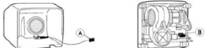
Means for disconnection with contact separations at least 3 mm. (0,12") must be incorporated in the fixed wiring.
