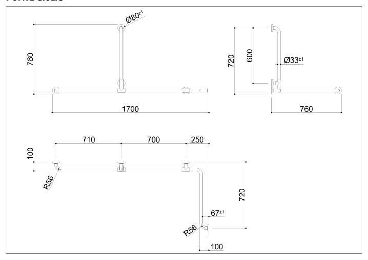
Corner and vertical grab bar made of zinc-plated steel pipe, coated with biocompatible and warm-to-the-touch vinyl
