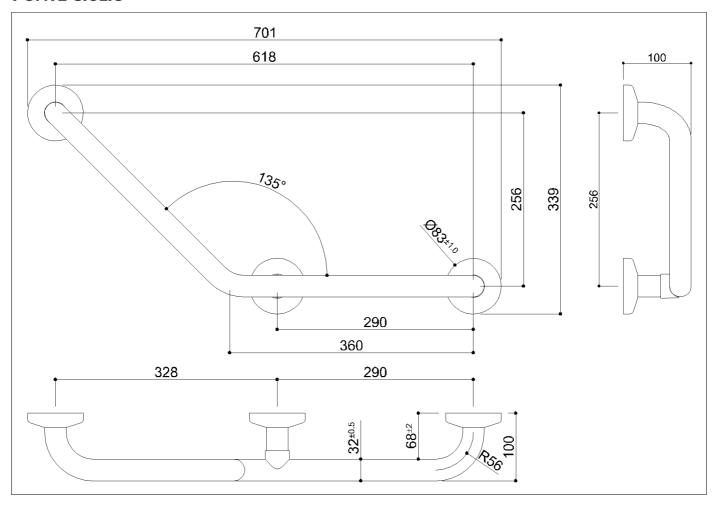
135° angled grab bar made of seamless steel pipe, painted with synthetic thermoplastic powder.
