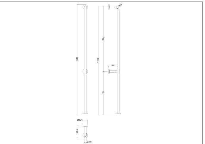
Wall-to-floor vertical grab bar made of zinc-plated steel pipe, coated with biocompatible and warm-to-the-touch vinyl
