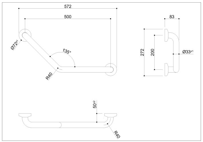
Safety corner grab rail  $135^{\circ}$  Ø 33mm with antislip, vinyl coating and zincplated steel internal pipe without junctions. Active and long lasting antimicrobial
