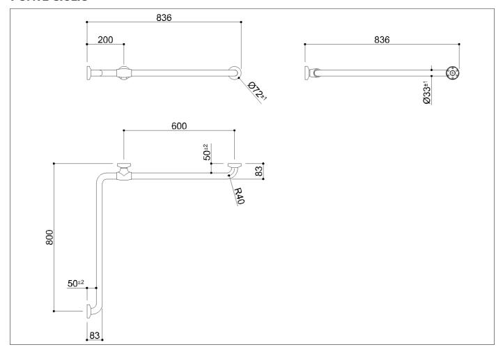
Safety handrail Ø 33 mm with vinyl coating and zinc-plated steel internal tube. Antislip coating, no junctions. Active and long lasting antimicrobial protection based on silver ions. Concealed wall clearance 50 mm. Wall fixing kit Ø 72 mm.. Fit for installation in bath and shower areas to enable the person to grab for standing and elevating from lower positon. Left or right
