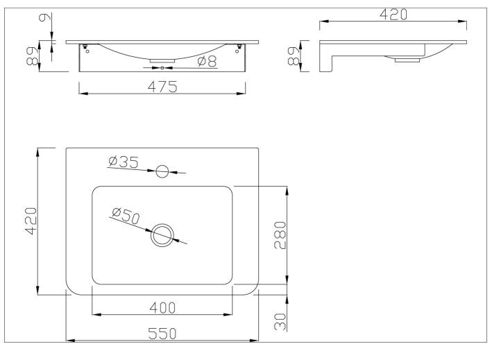
White acrylic stone rectangular console. This article can be customised on request as far as sizes and shapes. Particularly suitable for children school installation. The item is equipped with a white epoxy powder painted steel structure for wall fixing.
