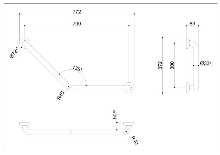
Safety corner grab rail 135° Ø 33 mm with antislip, vinyl coating and zinc-plated steel internal pipe without junctions. Active and long lasting antimicrobial
