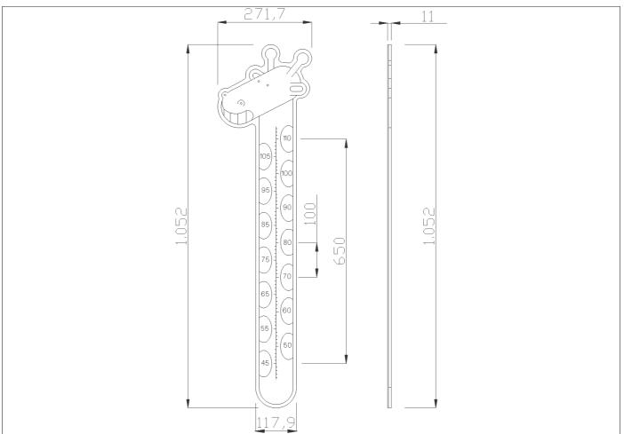
Giraffe neck-shaped HPL board, 12 mm thickness, with engraved decoration for height measurement of the children. The board is only in light blue colour with contrasting blue elements.
