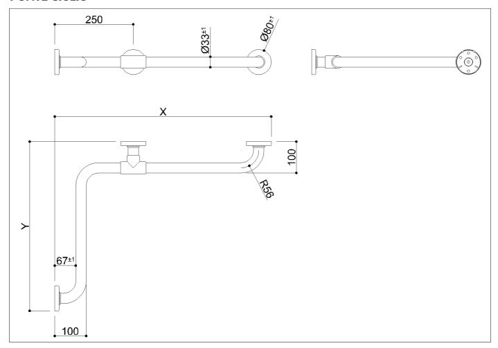
Customised corner grab bar made of zinc-plated steel pipe, coated with biocompatible and warm-to-the-touch vinyl.
