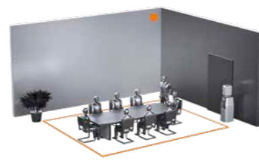
Conference-room situation, detection by the HPD2. Number of persons is detected.
