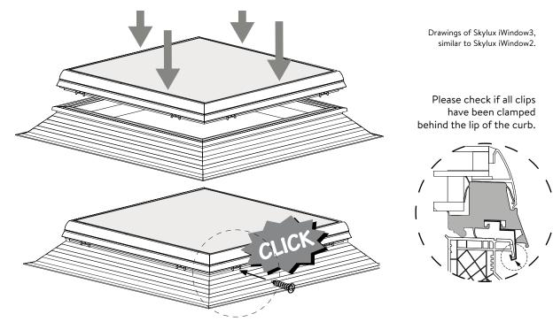
For extra reinforcement, screw the clips through the curb with delivered screws.
