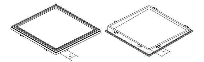
Attach the upper hinges of the frame to the lower hinges of the sloping PVC frame 08/00.
