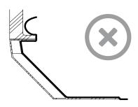
**Incorrect:** roof covering is pulled up over the flange
