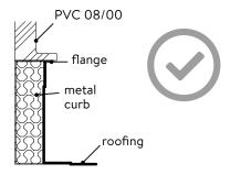
**OK:** roof covering is pulled up to below the flange
