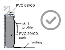
OK: roof covering is pulled up to below the skirt profile
