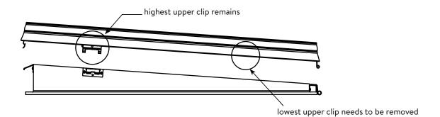
Check if the position of the upper clips matches the position of the lower clips. Move the upper clips if necessary.
