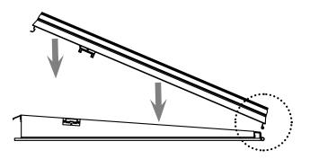
Insert the threaded rod with the mushroom heads into the hinges and use Loctite.
