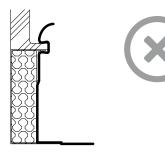
**Incorrect:** roof covering is pulled up over the flange
