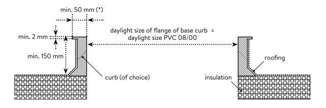
(\*) Max. 60 mm for daylight sizes with short side > 1,000 mm, because the hinges are located here.
