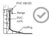
**OK:** roof covering is pulled up to below the flange
