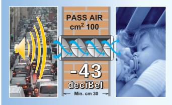
Helix43 is an acoustic reducer for ventilation holes in the external walls and/or ventilation duct. Available items allow to have a noise reduction of 43 decibels maintaining a section of air passage of 100 cm². It is recommended to use "La Ventilazione" grilles with certified air passage.
