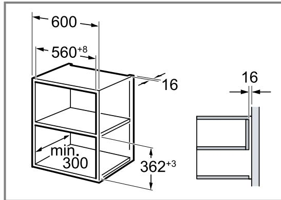
Do not fit the appliance too high up; it must be possible for accessories to be removed easily.
