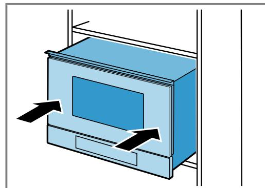
Do not kink or trap the connection cable, or route it over sharp edges.
